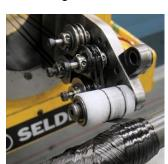
Only the highest grade of pre-pre carbon fibre are used to give sailors the best stiffness-to-weight-spar. The pre-preg carbon tows are UV stabilised to give a guaranteed long life, even in the sunniest of climates.
